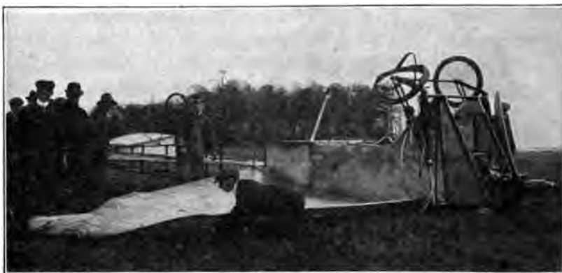
Fig. 47. Overturned Monoplane Due to a Start in a Gale
